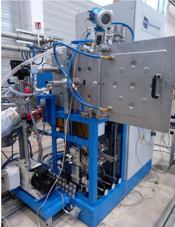
Test furnace with carbon xerogel door insulation © Aerofurnace funded by BMWK, project number 03ET1503 A-C
